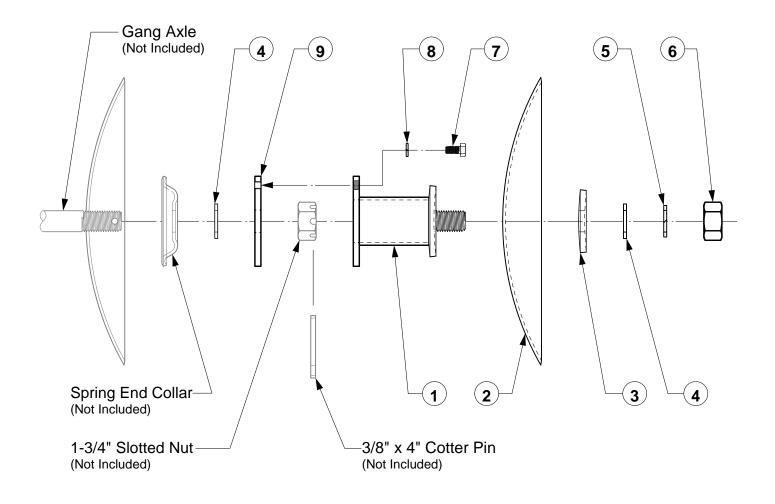
Note: Items "Not Included" are mounted on end of each disc gang axle.
